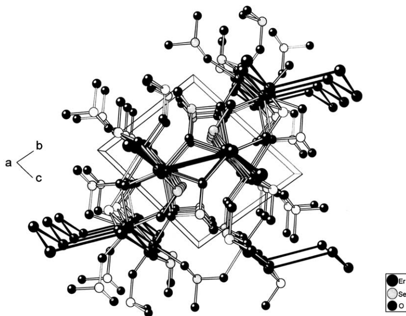
FIG. 3. Arrangement of the \text{Er}^{3+} ions in the crystal structure of \text{Er}_2(\text{SeO}_3)_3 . Chains of edge-connected chairs are formed which extend in the [100] direction.
